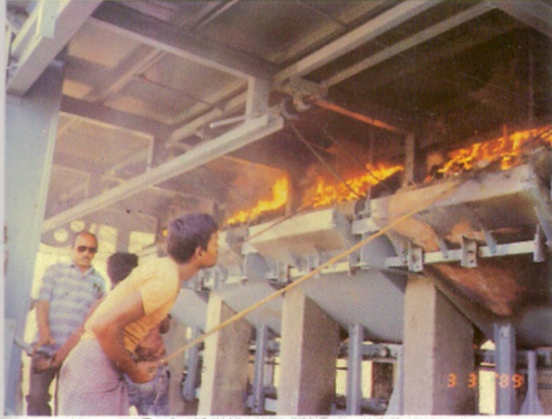
Retorts in Operation (Coke discharge)
