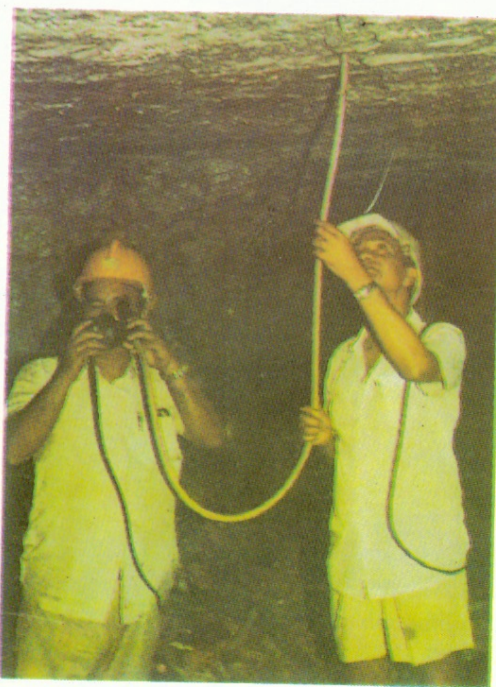
Fibre optic stratascope to determine bedding characteristics of roof rocks
