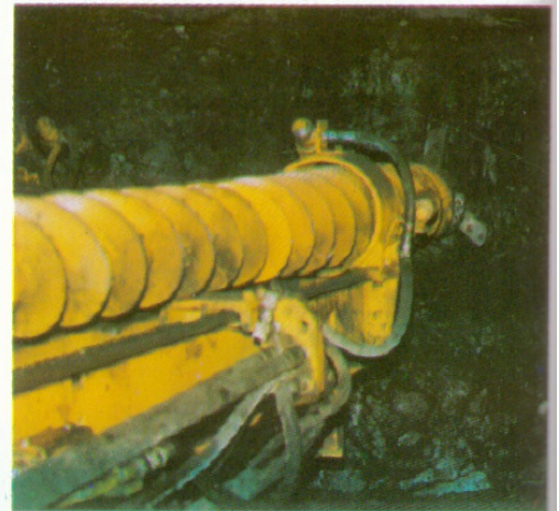
Auger-cum-drill at Coal face
