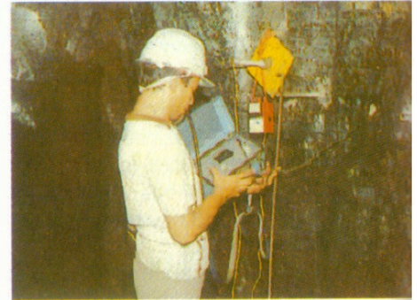
Stress and Deformation study with vibrat wire stress capsule and Borehole Extensometer
